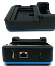
1-slot ethernet / USB host cradle with spare battery charging compartment and PSU (US/UK/EU adapter) 5000-900059G
